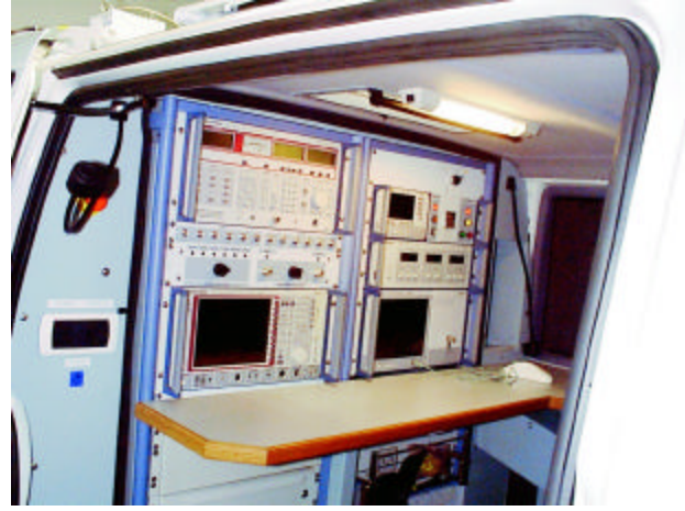
The Radiomonitoring/Location and Coverage van is equipped with a spectrum analyzer up to 26.5 GHz, a direction finder and a mobile coverage test system for digital networks. In order to cover a broad frequency range, different antennas are available, including an antenna mast.
