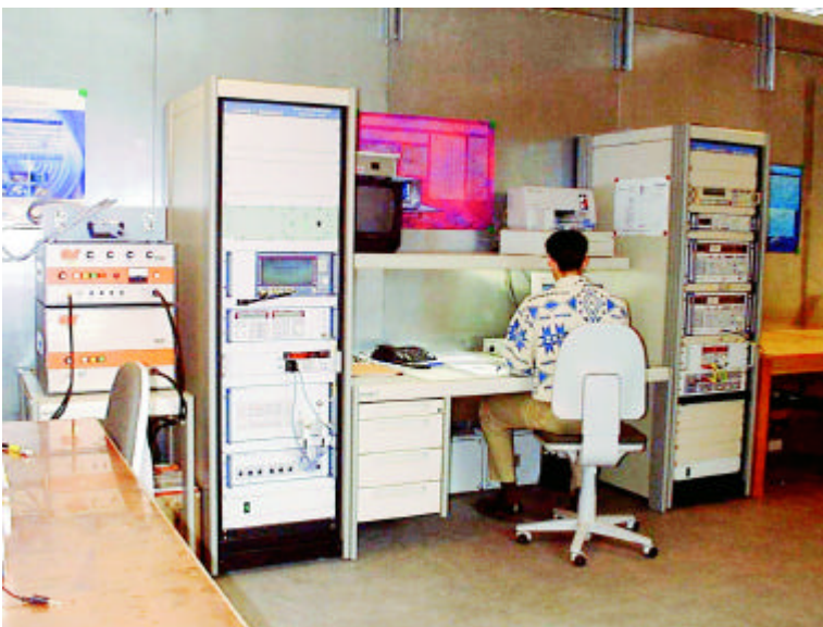
The EMC Centre of SEE in Luxembourg allows full conformity EMC testing up to 1 GHz, with ETSI tests on analog equipment.
