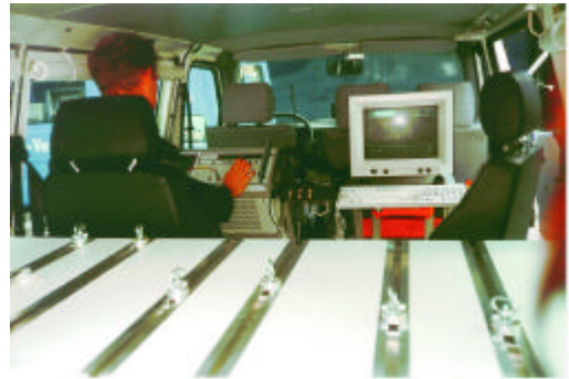
Inside view of a van for measuring field strengths.
