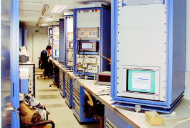
A complete mobile calibration van for automatic calibration of RF and LF instruments and passive devices.
