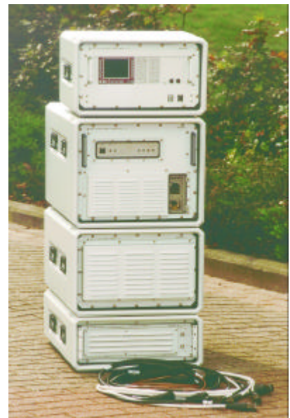
10 HF transceivers with ALE-capability transformed for IP54 intrusion protection and built into special transport cases.
