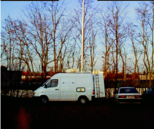
Test vehicle for broadcast radio and TV transmission measurements (UHF, VHF)
