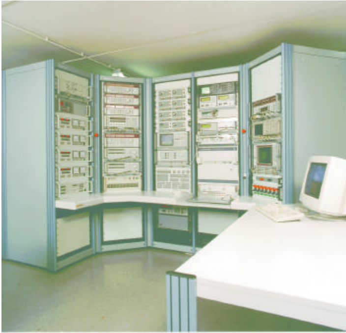
Full automatic repair and maintenance system for telecommunication equipment.
