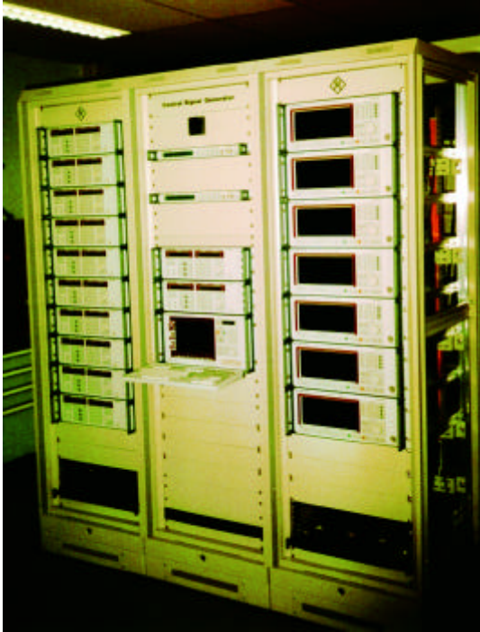
Test system for distribution of calibrated 9 AM and 10 FM signals with RDS for testing car radio tuners in production
