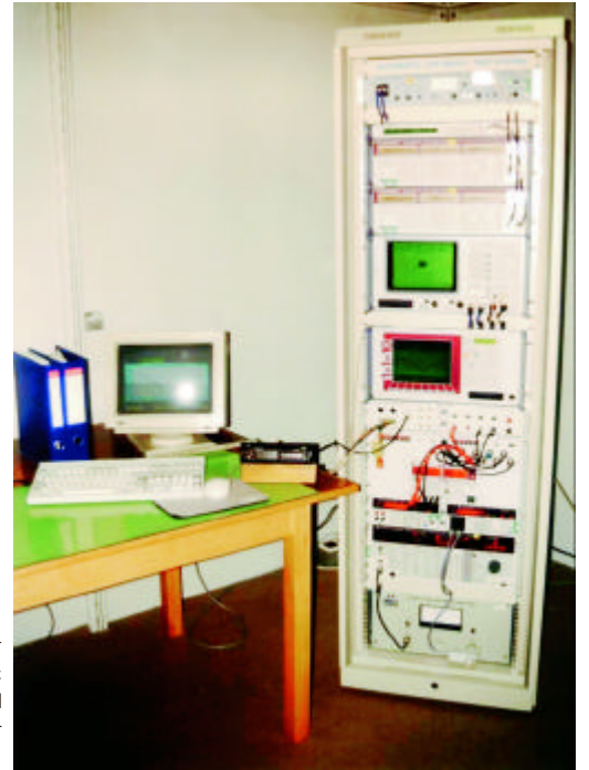
Test system for automatic measurement of all audio- and RF car radio parameters.
