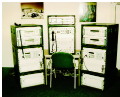
Two HF 400 W transceivers and four HF receivers built into special transport cases.
