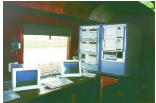
Test system for the control and real-time measurement of RF-radio links, with a special data logging and processing software, built into a carriage.
