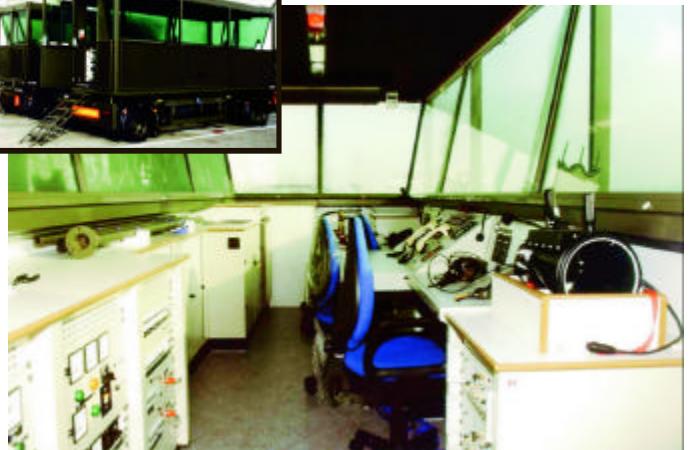
Mobile Air Traffic Control Tower equipped with a complete communication and meteo system, transportable by a C130 aircraft.
