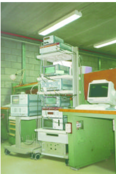
Automatic test system for full automatic calibration of R&S radiocommunication testers like CMS and CMT.
